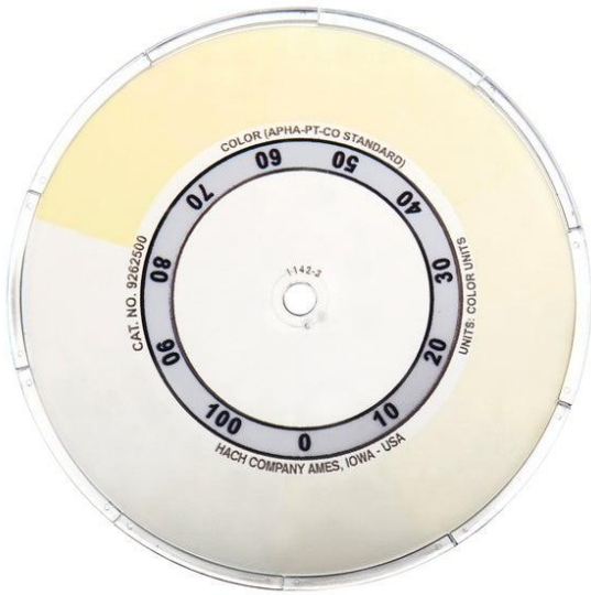
Figure 43. Hach CO-1 comparator disc calibrated in Platinum-Cobalt units
